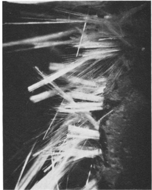
Figure 5 A micrograph illustrating a combination of pull out and fracture of fibres at failure ( \times 60 ).
